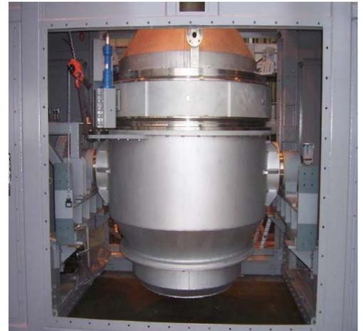
The Static Detonation Chamber
